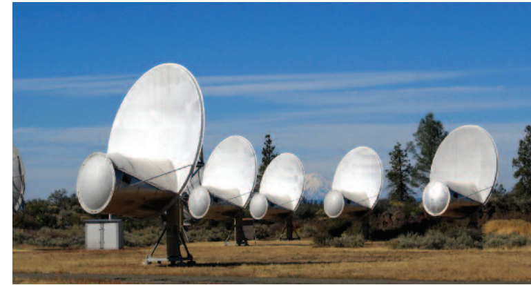
▲ Hat Creek Allen Telescope Array, the "Alien Telescope Array", California, USA. These radio telescope 6-metre dishes are used in the Search for Extraterrestrial Intelligence (SETI).
